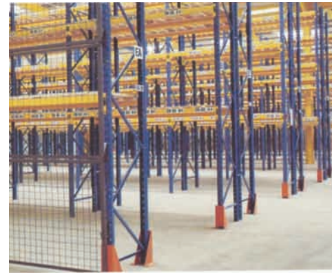
Column guards and mesh screens.
